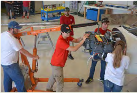
From left, Erie 1 BOCES Aviation Technology students Christopher Kozak, Aidan Hurley, Jacob Bell and Tatiana Forbes work to install an engine on the Sportsman 2+2 airplane.
